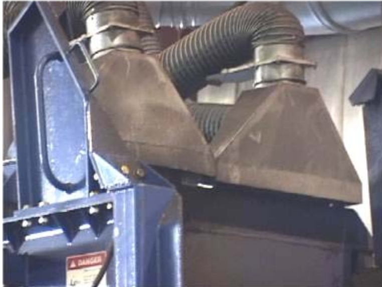
Picture 18 - Pneumatic Dust Control System Added on to a Standard Shingle Grinder
